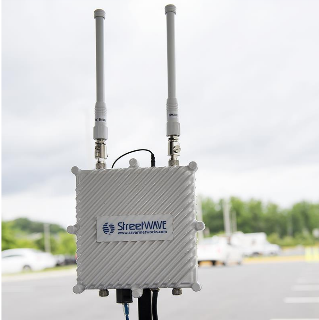
DSRC Roadside Unit (RSU)
