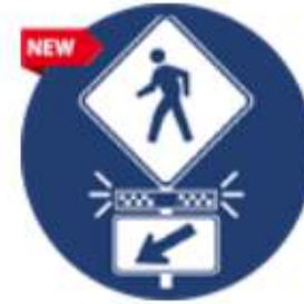
Rectangular Rapid Flashing Beacons
