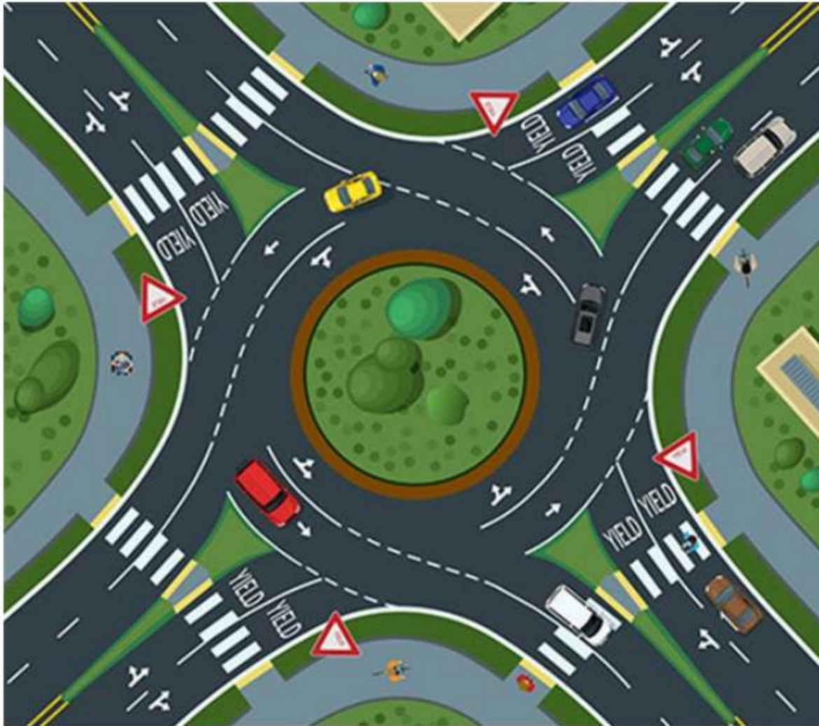
Illustration of a multi-lane roundabout. Source: FHWA
